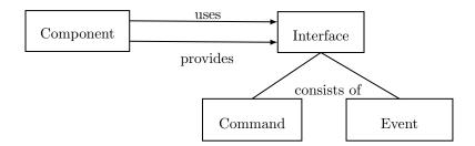
Figure 2.5: NesC components and interfaces
