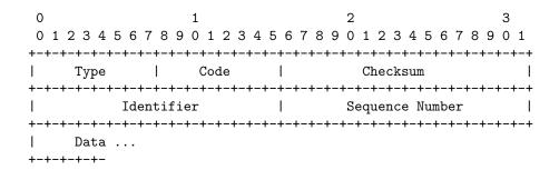
Figure 3.4: ICMPv6 Echo Request and Echo Reply message format
