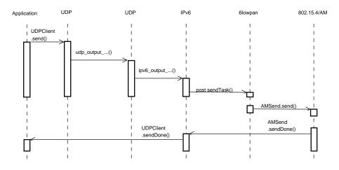
Figure 4.3: Sending a UDP packet
