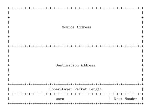
Figure 3.2: IPv6 pseudo-header for upper-layer checksum computation
