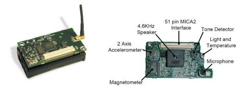
Figure 2.2: MicaZ mote [11] and the MTS 310 sensorboard [13]
