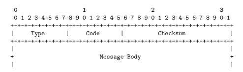
Figure 3.3: ICMPv6 general header format
